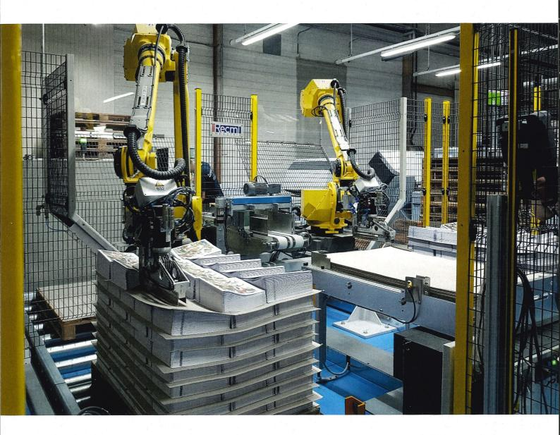
Robotic palletizing for high-speed folder deliveries / finishing lines
