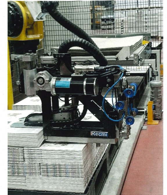
Guiding the pile from pick-up to laying on the pallet
