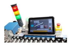
Robot configuration software allows the operator to design quickly a new pallet pattern or load an existing one thanks to the touch screen (tablet) configuration.
