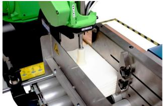
No changeover, the specific tool ensures a precise taking-off and droping of the various stack formats, preserving the products.
