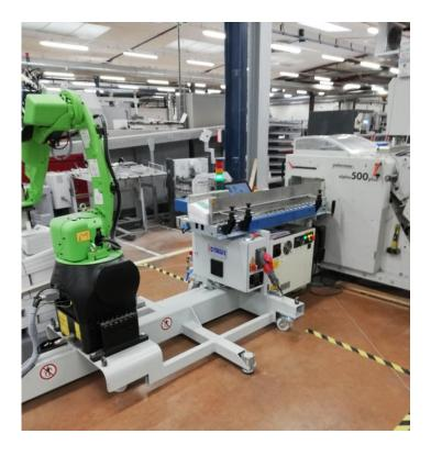
The new RECMI collaborative robot palletizer is designed to palletize a large range of products from folder deliveries and end of lines: folded signatures, saddle-stitching, sealed binding ....
